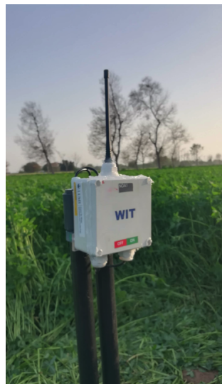
Figure 3: Sensors (Air) and Transmitter Attached to the Pole
